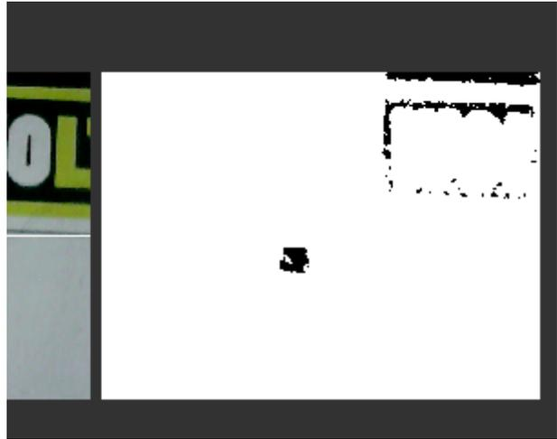
*Example of bad contrast setting. The marker recognition will fail if the contrast is not corrected.*
