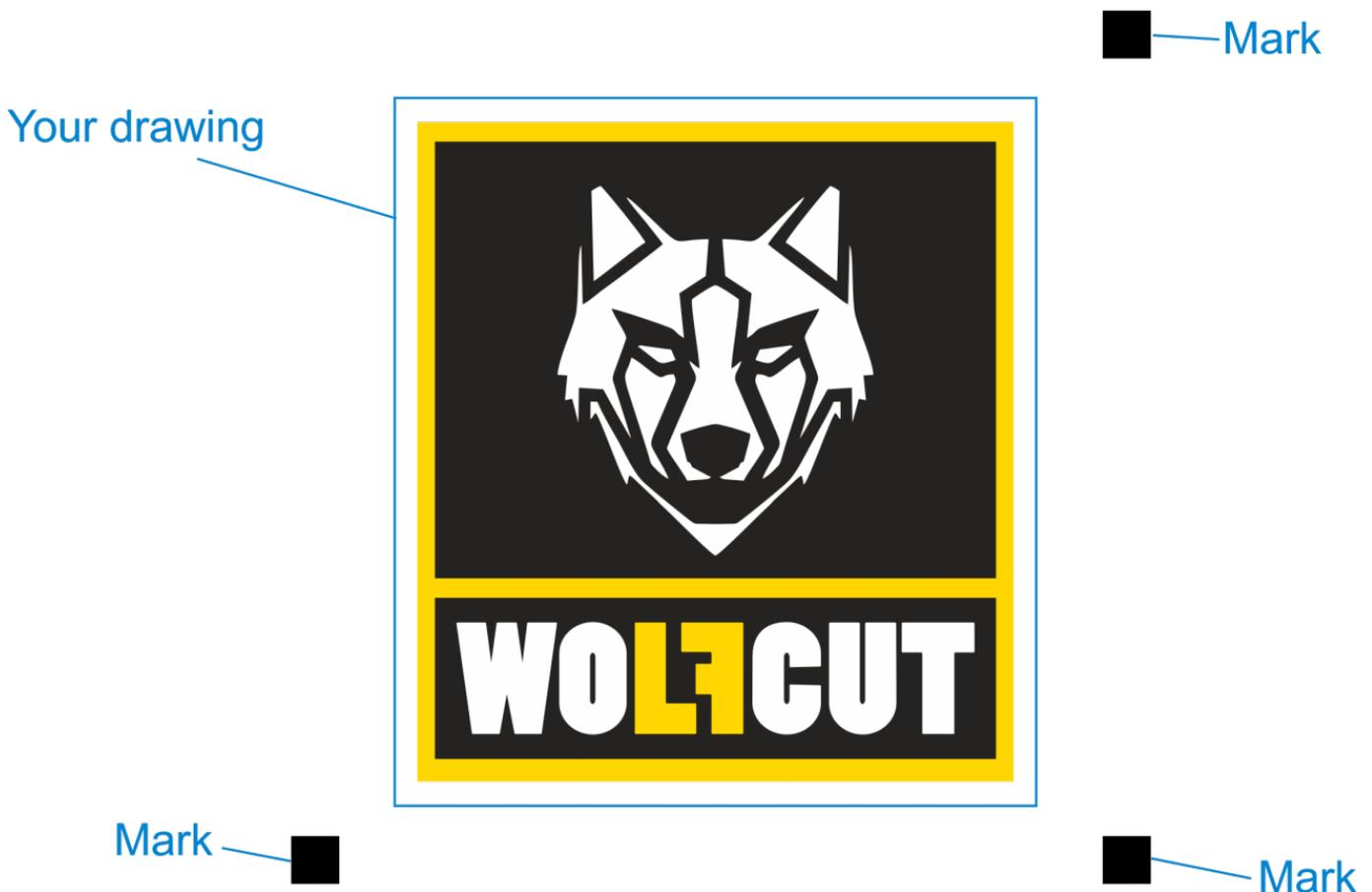
*Recognition marks on the printed drawing, these marks will be visible to the camera.*
