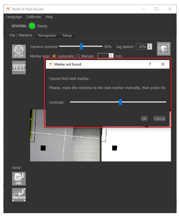
To continue the recognition you need to manually move the CNC machine so that the camera is over to the mark then click "OK" (or use the cursor keys and press enter...).
